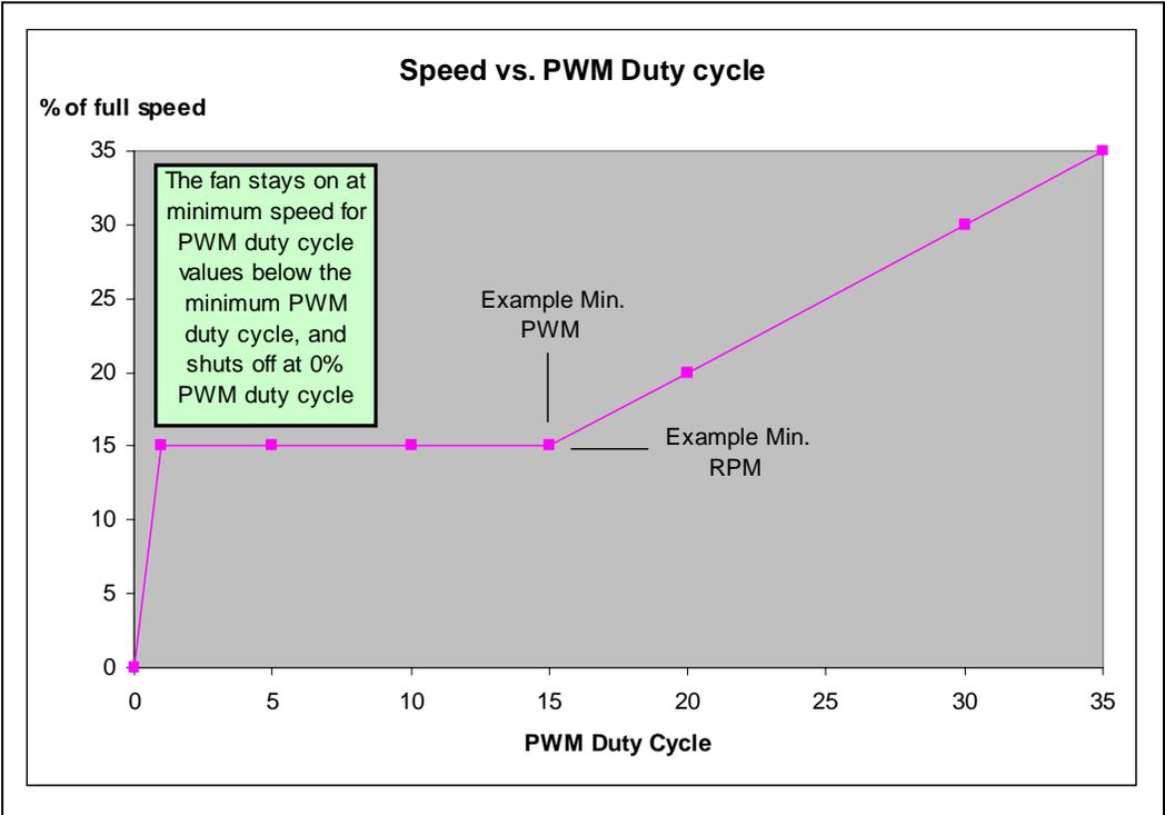
In Type C implementation the fan will stop running when the current provided to the motor windings is insufficient to support commutation. The fan should not be damaged from this. The fan would also turn off the motor at 0% PWM duty cycle input. See Figure 5.
